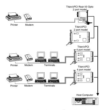
Figure 6: 10-port configuration using Front and Rear I/O
